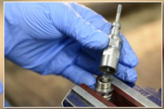
• HOLD THE KEY DRIVE END AND TWIST THE MOLE GRIPS IN AN ANTI-CLOCKWISE UNTIL CABLE HEAD IS DETATCHED
