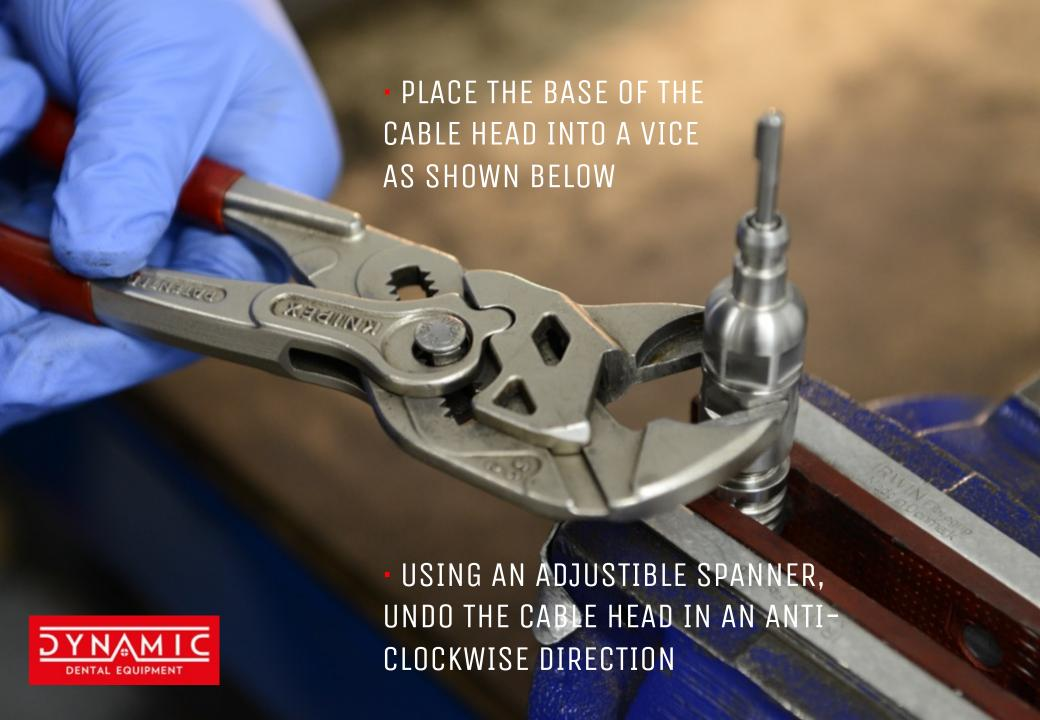
• ONCE THE CABLE HEAD IS UNDONE, STRETCH THE CABLE HEAD SO THE INNER CABLE IS EXPOSED. THEN ATTACH THE SMALL MOLE GRIPS TO THE INNER CABLE WHICH IS EXPOSED.
