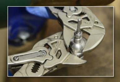
• USING TWO ADJUSTIBLE SPANNERS, DISMANTLE THE CABLE HEAD AS SHOWN IN PICTURE
