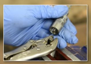
• HOLD THE SQUARE DRIVE END AND TWIST THE MOLE GRIPS IN AN ANTI-CLOCKWISE UNTIL CABLE HEAD IS DETATCHED
