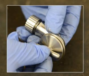
• ATTACH HEAD BACK ONTO THE SHAFT BY TIGHTENING THE NUT ON THE TOP OF THE SHAFT IN A CLOCKWISE DIRECTION. TAKING CARE NOT TO CROSS THREAD.
