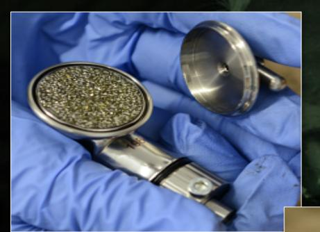
PLACE THE DISCREMOVAL TOOL OVERTHE DISC
