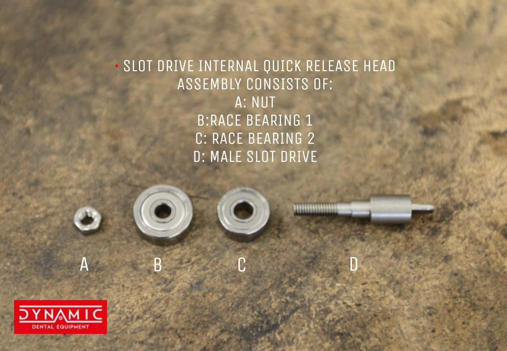
REPLACE BEARINGS B AND C AND THEN DO UP THE SLOT DRIVE INTERNAL ASSEMBLY
