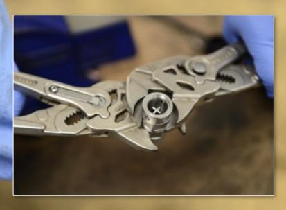
THEN USING TWO 18MM SPANNERS TO DISMANTLE CABLE HEAD, UNDO IN AN ANTICLOCKWISE DIRECTION AS SHOWN PICTURE
